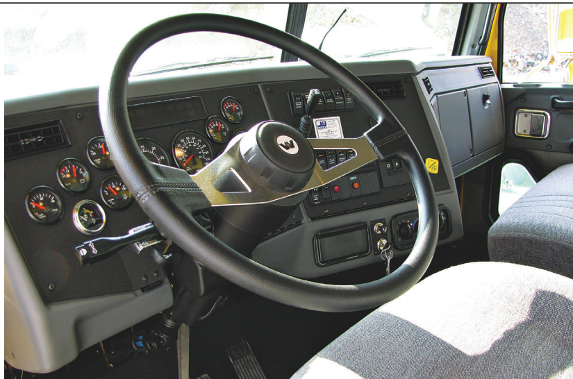
Cab is from 4900 series and its gauges and controls are similar. Controls include switches for Jake Brake and a lever for the Allison's hydraulic retarder.
