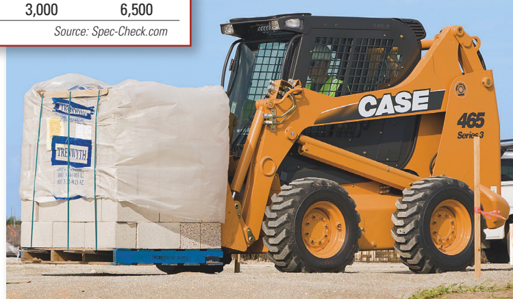
Arm-lifting force increased on four of the eight Case 400 Series 3 skid steers, including a 12-percent boost for the 3,000-pound-rated 465.
