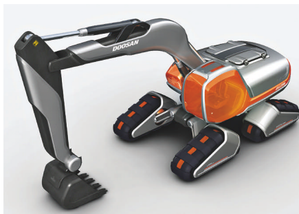
Doosan's CX concept excavator rides on four swing arms with independent tracks.
