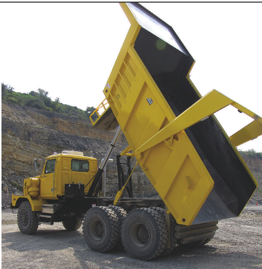
Stout J&J body is made of Hardox steel, and hoist tips it in 25 seconds at 1,000-rpm engine speed, according to specs. Tailgate stays stationary during dumping.
