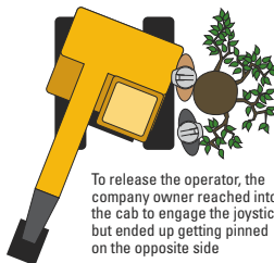
As the operator exited the cab without locking the interlocking lever, the cab turned and pinned him against the tree
