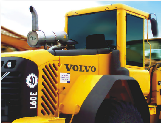
Volvo entered a partnership with Huss to provide exhaust retrofits for Volvo equipment that significantly reduce diesel emissions.
